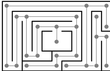
Figure 3.1: Maze with waypoints represented by dots.
