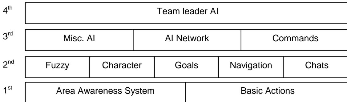
Figure 5.1: Layered architecture
