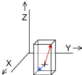
Figure 6.3: 'mins' and 'maxs' vector in bounding box.
