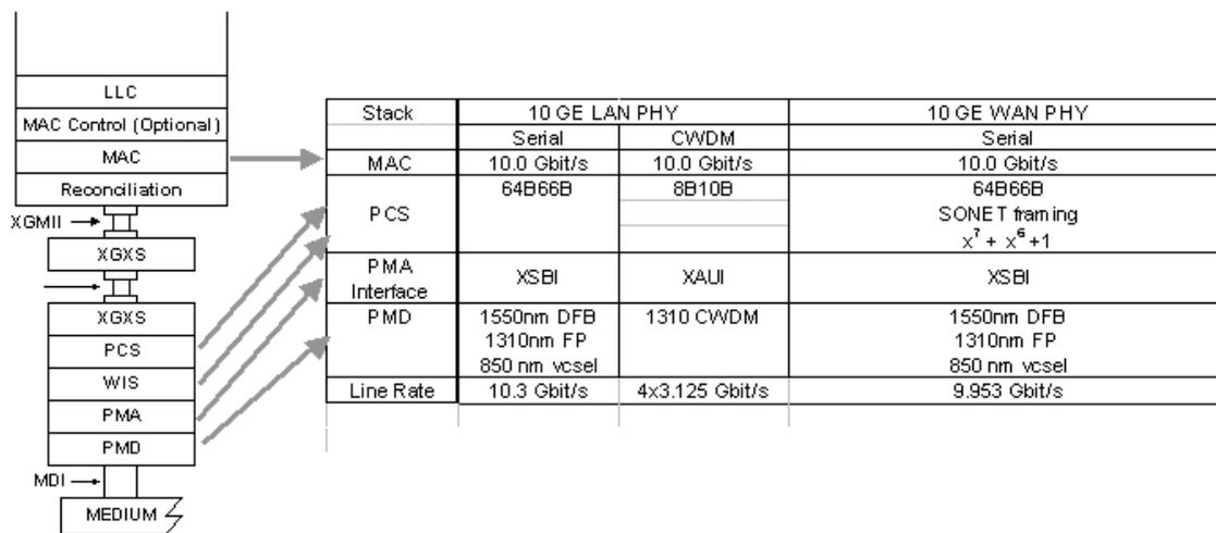
Figure 8. Detailed Illustration of the LAN and WAN PHYs and associated PMDs.
