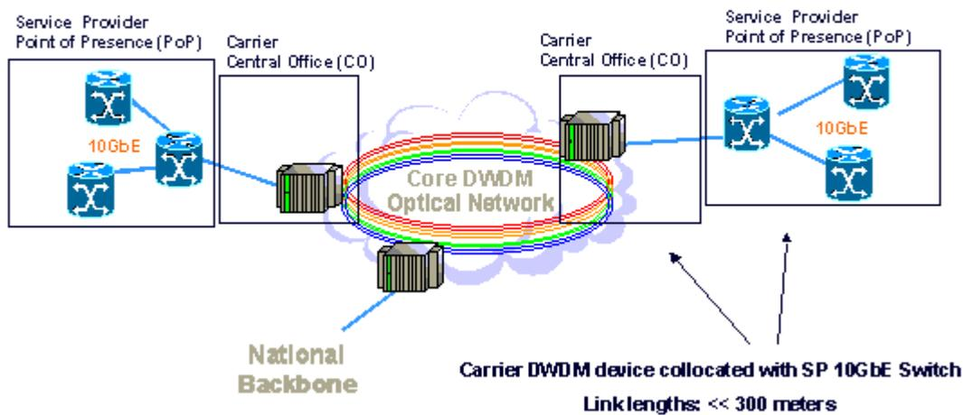
Figure 12. Example of 10 Gigabit Ethernet in WAN applications.
