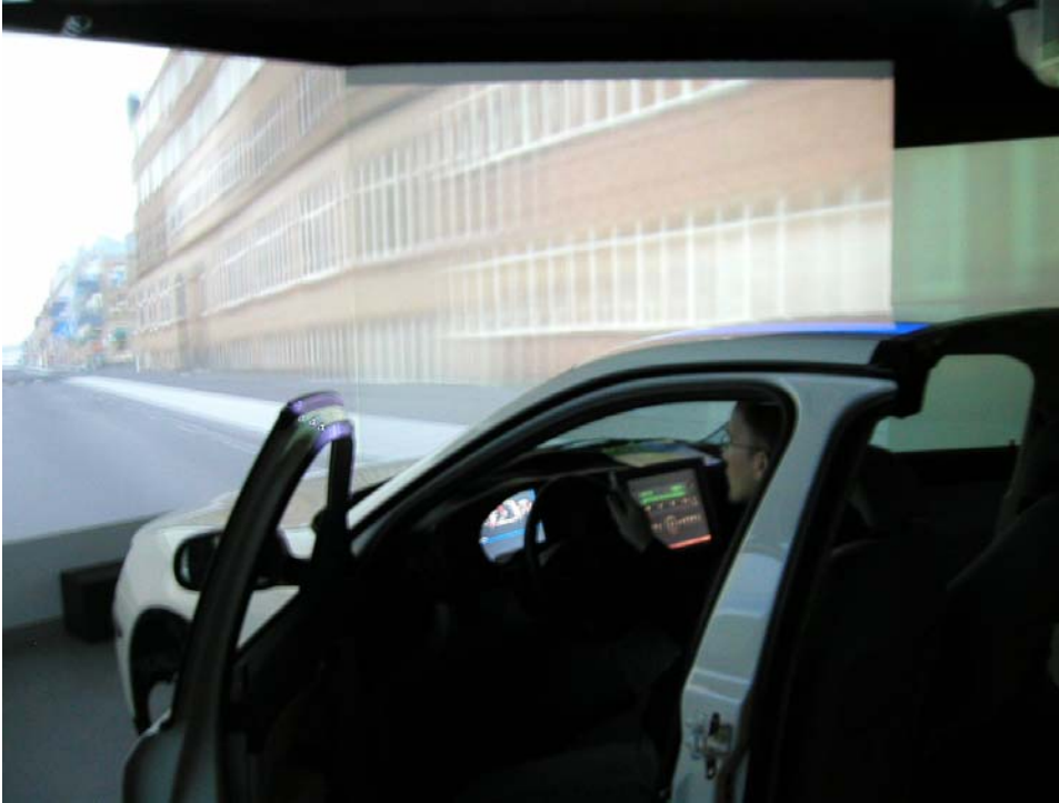
Figure 3. The Saab cockpit and the visual scene in the Driving simulator at Linköping University.
