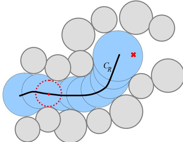
Fig. 4.1: Atoms (gray circles), tunnel (blue circles), tunnel centerline  $C_R$  (thick black line), bottleneck circle and bottleneck point (red dotted circle and its center), active place (red cross).
