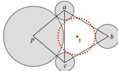
Fig. 5.4: The center of the circle  $s$  lies in the orthogonal center of a triangle  $abc$ . The circle  $s$  does not have any intersection with the atoms  $a$ ,  $b$ ,  $c$ , but it still intersects the atom  $p$ .
