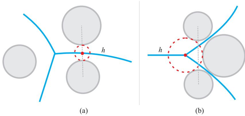
Fig. 5.2: (a) The bottleneck point (dashed circle) of  $h$  lies in the point of intersection of the edge  $h$  and the plane passing through neighboring atoms, (b) The bottleneck point in the endpoint of  $h$ .
