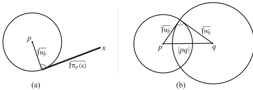
Fig. 3.2: (a) Power distance, (b) Two orthogonal weighted points.
