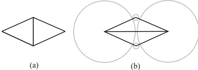
Fig. 3.1: (a) Delaunay triangulation (in 2D), (b) Regular triangulation (in 2D). The circles represent weights of the points.
