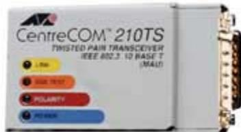
When this transceiver is correctly connected, the “POWER” LED should light. Similarly, the “LINK” and “POLARITY” LEDs should light when you inserted the cable into the RJ45 socket on the transceiver. (Note that to get this result; the other end of the cable should be connected to some other devices as well.) If these LEDs are not light, you probably have problems with the link (cable).
