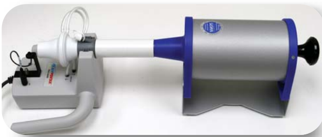
A one-liter syringe is provided for calibration to ensure accurate measurements.
