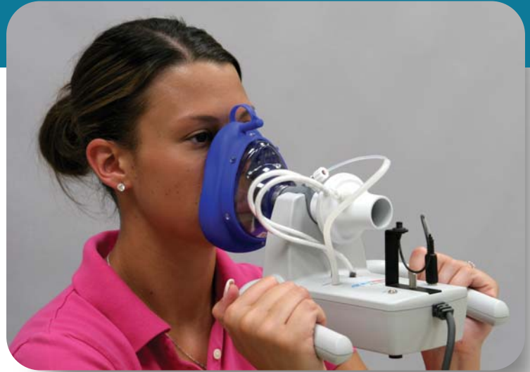
Using the dual handles, the client holds the PAS mask up to the face during data collection.
