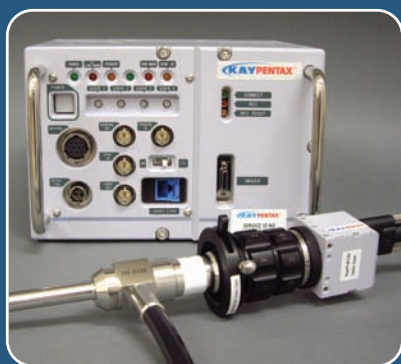
The High-Speed Camera Controller and color camera head, with lens adapter and rigid endoscope. Camera head dimensions are 35 mm x 35 mm x 35 mm and weight is 90 g (3.2 oz).
