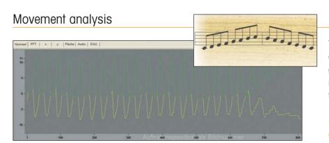
The movement of the vocal cords can also be analysed in the form of a glottogram. The user defines regions of interest, the dynamics of which are then plotted as a curve.
