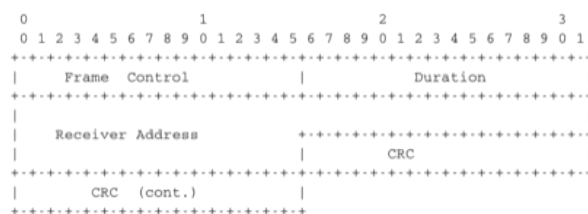
Fig. 3.98: IEEE 802.11 ACK and CTS frames
