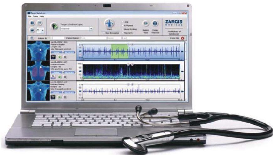
FIGURE 9.32 The Littman Electronic Stethoscope uses Bluetooth v4 to transmit sounds in real time to a Laptop for further analysis. (Courtesy of eweek.com).
