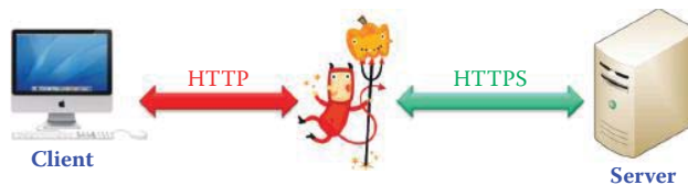
FIGURE 23.6 Man-in-the-middle uses the HTTP to capture a password and logs in using the password captured. The client can read the relayed https message that was decrypted by the middle man.
