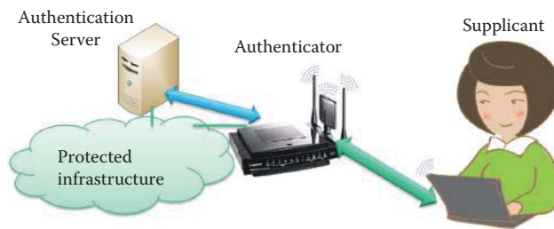
FIGURE 25.14 The 802.1X structure for controlling a host when connecting to a LAN.
