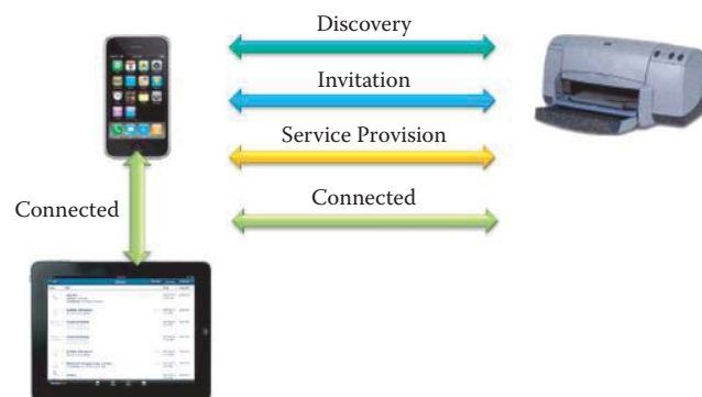
FIGURE 5.13 The P2P Invitational Procedure enables a Wi-Fi Direct device (a printer) to become a P2P Client of an existing P2P Group.
