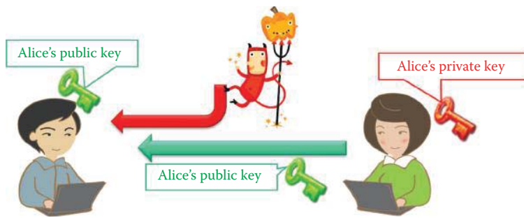
FIGURE 22.1 The public key concept: Alice has a key pair; Alice wants everyone to know her public key, but the private key is known only by her.
