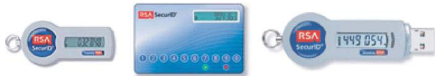
FIGURE 20.13 RSA SecurIDor tokens that provide one-time passwords. (Courtesy of RSA Security.) The left one is designed for a user to type the passcode displayed on the token; the center one allows a user to type in a PIN to the token and then a passcode will be generated for a user to type into a computer or smart phone. The right one has a USB interface and can send a password directly to a computer.
