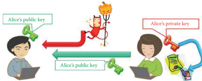
FIGURE 22.4 The digital signature concept: Alice provides a signature using her private key, and it can be verified since everyone knows her public key.
