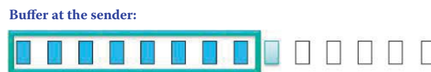
FIGURE 15.15 The window is full now and one byte remains to be sent.
