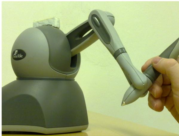
Figure 6.1: The haptic device Phantom Omni<sup>®</sup> used in our lab.
