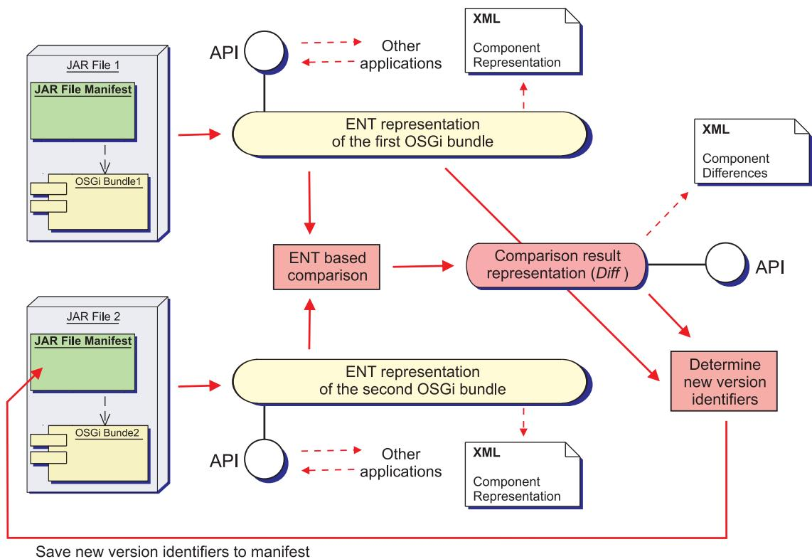
Figure 3: Schema of the comparison algorithm
