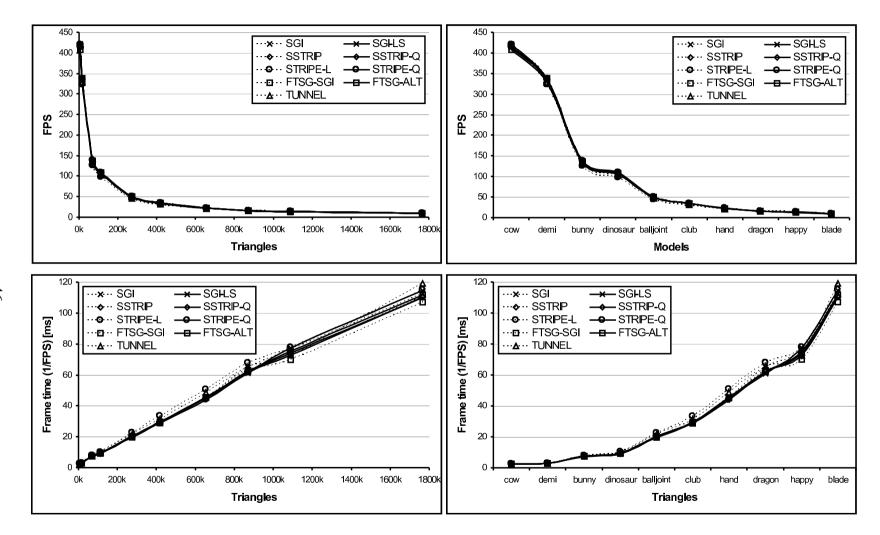
Figure 3.22: Graphs: Average FPS (top). Rendering time for a single frame (bottom).
