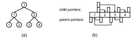
Figure 3.18: An example of a merge tree (a) and its corresponding skip list structure (b). (From [13])
