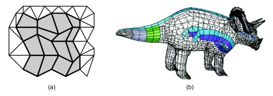
Figure 3.5: An example of a rectangular patch (a) and a typical polyhedral mesh with patches (b). (From [16])
