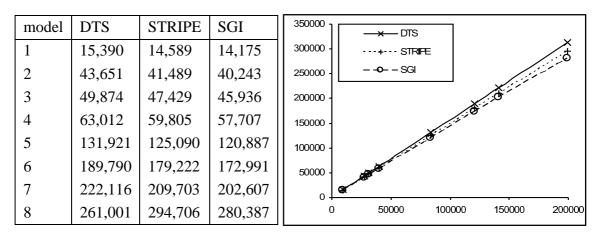
Table 4.5 lists the number of vertices in strips for all algorithms. The *DTS* algorithm produces 5–6% more vertices than the *STRIPE* and 8–11% more vertices than the *SGI*.
