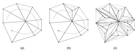
Figure 3.14: The initial triangulation contains the convex hull and one inner point (a). While inserting the remaining vertices, the strip can be preserved (b). The final triangulation contains only one strip (c). (From [3])
