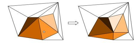
Figure 4.11: Insertion of a vertex changes the order of triangles (the color intensity marks out the order of triangles).
