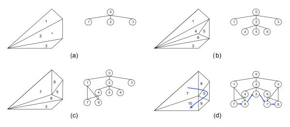
Figure 4.2: Example of DAG. A new point is inserted into a triangulation (a). The corresponding triangle is subdivided into three new triangles (b). The triangles checked for the Delaunay condition (c) and (d).
