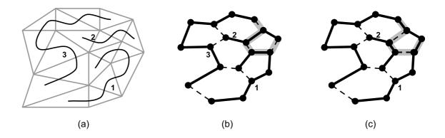
Figure 3.10: A triangle mesh with three strips (a). The tunnel (gray) is an alternating sequence of strip (solid) and nonstrip (dashed) edges (b). Complementing the status of edges in the tunnel, the number of strips is reduced by one (c). (From [32])
