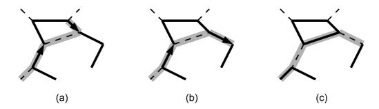
Figure 3.12: If a nonstrip edge connects two strip edges of the same strip, the orientation of those edges toward the end of strip has to be opposite (a). If this condition is not fulfilled (b) an infinite loop appears (c). (From [32])
