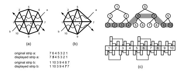
Figure 3.19: An original mesh covered by two strips (a), A decimated mesh (b) and corresponding merge tree and skip list (c). The dark area in the merge tree shows the active LOD for the mesh. (From [13])
