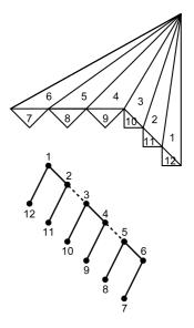
Figure 3.6: FSTG algorithm steps and an example of a triangulation and its corresponding dual graph. (From [39])
