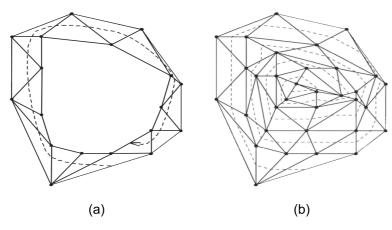
Figure 3.15: The annulus bounded by the first and the second convex hull is triangulated and a strip connecting all triangles is created (a). Following the same construction scheme, the whole triangulation can be created (b). (From [3])
