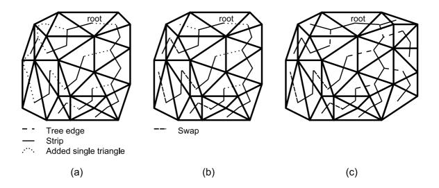
Figure 3.9: The basic traversal strictly maintains the left-right turn sequences. Some singleton strips can be added to existing strips even if there are not connected in the spanning tree (dotted line) (a). Relaxing the left-right turn criterion (allowing swaps – dense dashed line), the number of strips can be lowered (b). The strips can be extended in "wide" nodes (typically the root node) (c). (From [30])
