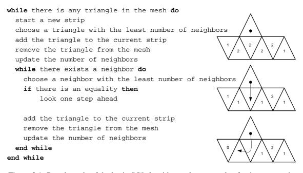
Figure 3.1: Pseudo-code of the basic SGI algorithm and an example of strip construction.
