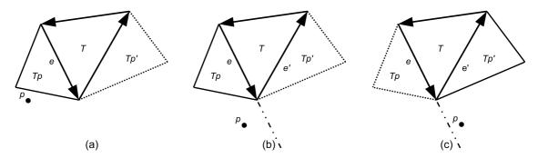
Figure 3.8: If the closest point to point p is an inner point of the edge e of the triangle T, then  $T_p$  is the predecessor of T (a). If the edge e is exposed to p, then  $T_p$  is the predecessor of T (b) else  $T'_p$  is predecessor of t (c). (From [30])
